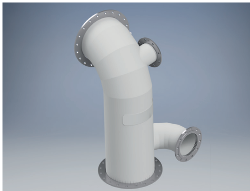
Water injection piece for a main engine, including relatively large bypass pipe.
